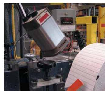
SG-300, Strobe Guard, Flex Arm SAS-DT-300, Flash Tubes and Sensors, shown in typical print inspection/ registration application.
